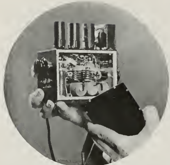
DEVELOPMENT MODEL OF INEXPENSIVE RADIO FREQUENCY CONVERTER WHICH ENABLES BLACK-AND-WHITE TELEVISION RECEIVERS TO REPRODUCE COLOR PROGRAMS IN MONOCHROME.
