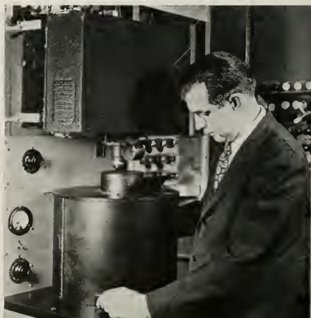
RAY D. KELL OF RCA LABORATORIES ADJUSTS THE ALL-ELECTRONIC COLOR CAMERA. THE CYLINDRICAL UNIT HOUSES THE SCANNING KINESCOPE. MIRRORS AND PHOTOCELLS WHICH CONVERT COLOR INTO ELECTRICAL SIGNALS ARE IN THE UPPER CABINET.
