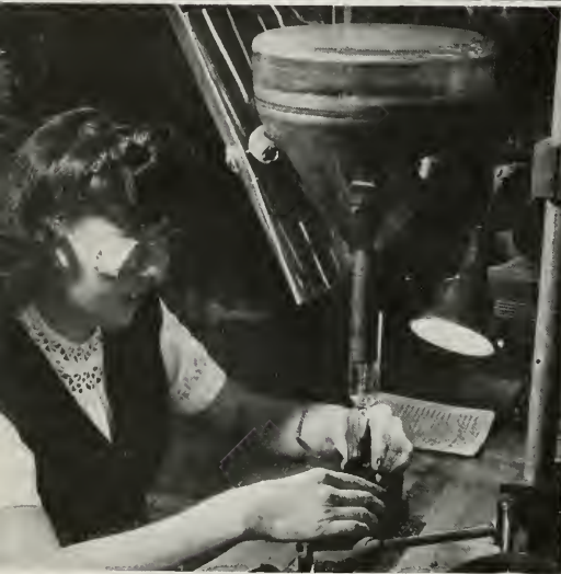
BELOW: NON-REFLECTING CARBON COATING IS APPLIED TO INTERIOR OF TUBE BY LONG-HANDED BRUSH TO KEEP STRAY ELECTRONS FROM THE PICTURE SCREEN.
